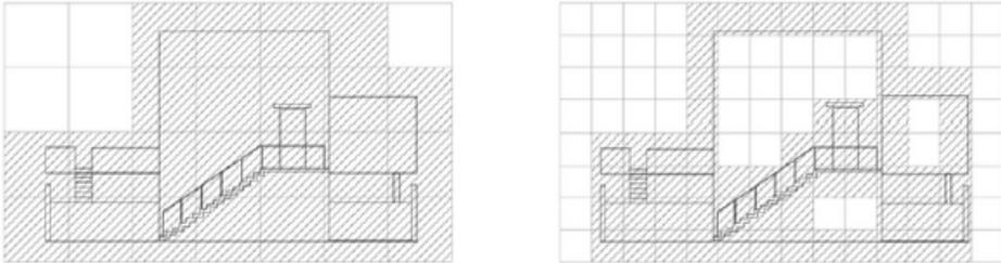
Figures 1 and 2: First Grid (Left) and Second Grid (Right) Placed Over Elevation 1 of the Y-House Showing Box-counting
